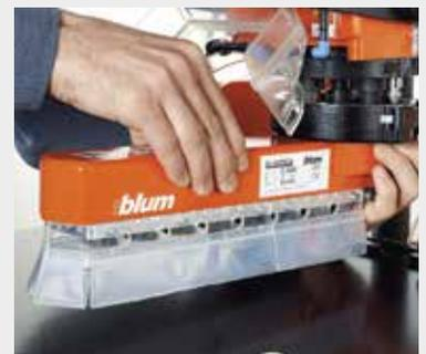
8 spindle drilling head: MZK.880S
